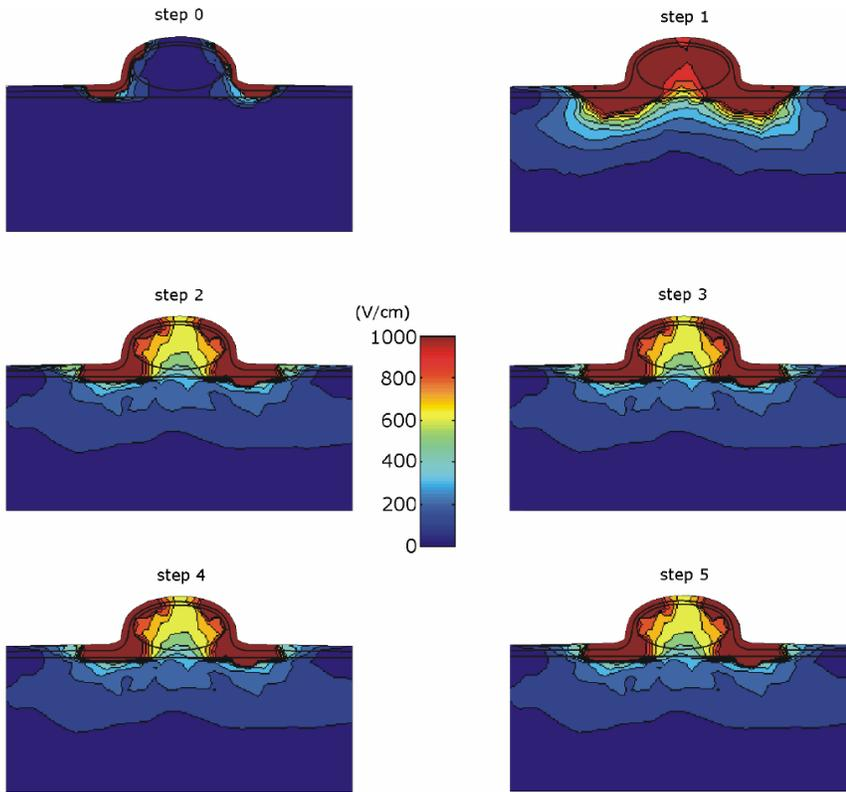
**Figure 5.** Six steps of the sequential analysis of the electroporation process in the subcutaneous tumor model at 1000 V between two plate electrodes with distance of 8 mm. The electric field distribution is shown in V/cm.
