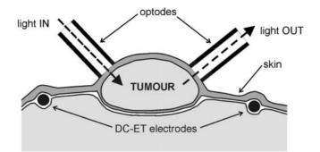
Figure 1. Experimental setup for NIRS measurements.
