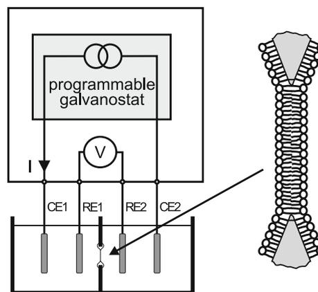
**Fig. 1** Measurement system with a programmable galvanostat and a voltmeter with four Ag–AgCl electrodes, two current electrodes (CE) and two reference electrodes (RE) plunged into the Teflon chamber compartments
