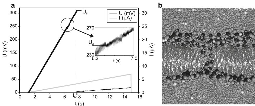
**Fig. 5** **a** Trace of the measured transmembrane voltage ( $U$ ) under linearly rising current ( $I$ ) conditions.  $U_{br}$  is the voltage at which bilayer breakdown occurs, and the *arrow* points at a transient voltage drop. After this event, the bilayer appears to recover completely
