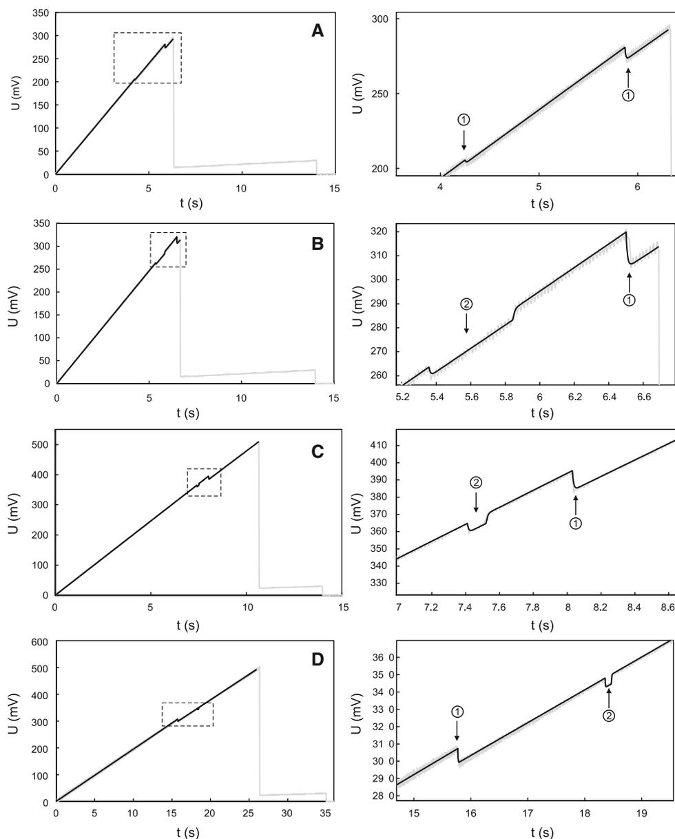
**Fig. 6** Experimentally obtained voltage traces (*light lines*) and best fits (*bold lines*) obtained with the SPICE model. The entire voltage traces are presented in the *left column* and a zoom on the event(s) on the *right*
