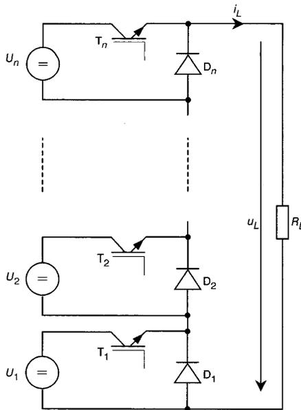
Fig. 1 Modular high voltage source
