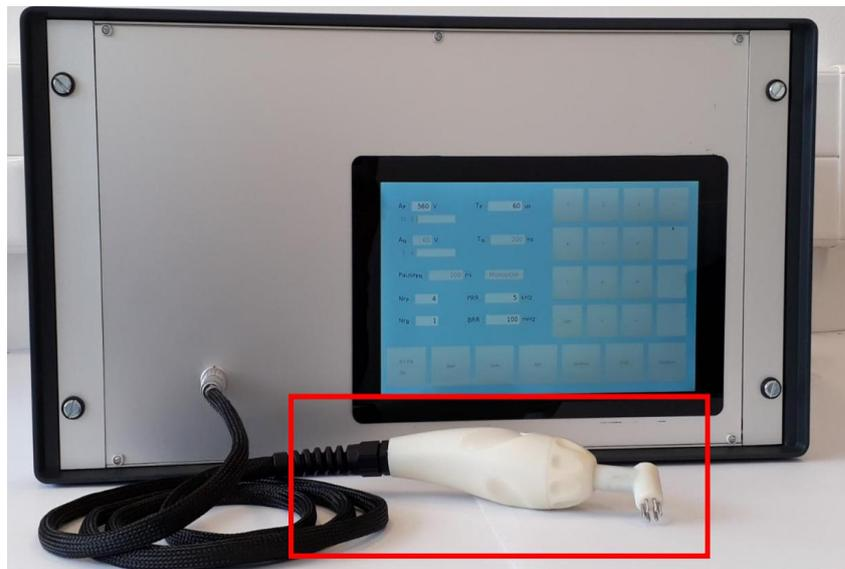
**Figure 5.** The completed device (pulse generator and applicator) for gene electrotransfer to skin cells. The applicator is shown inside the red frame.
