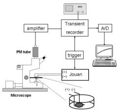
FIGURE 1 Schematic of the imaging system.
