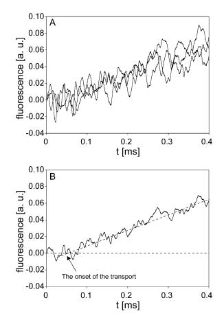
FIGURE 7 Onset of the transport of PI. (A) The time course of fluorescence increase obtained from three independent experiments. (B) Average of the three signals in A. CHO cells in suspension containing 1 mM PI were exposed to a single rectangular 1 ms, 800 V pulse. PM tube was set to the highest sensitivity, where all dynodes were activated. The background fluorescence was subtracted by the differential acquisition of the signal.
