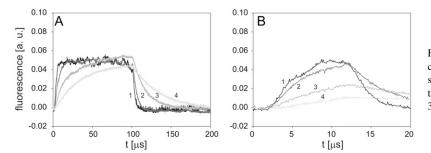
FIGURE 3 Time response of the imaging system on a step change of the light from a green LED. Durations of the LED signal were set to (*A*) 100  $\mu$ s, and (*B*) 10  $\mu$ s. Bandwidths of the amplifier: (*I*) 117 kHz, (2) 39 kHz, (3) 7.7 kHz, and (4) 3.5 kHz.
