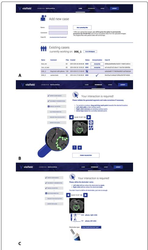
**Figure 5** The main working screens of the application. A. Cases (i.e. uploading images and selecting the active patient). B. Workspace (i.e. selecting the procedure, validating segmentation results, downloading final results, etc.). C. Electrode insertion module, in which electrode type and entry point can be specified.
