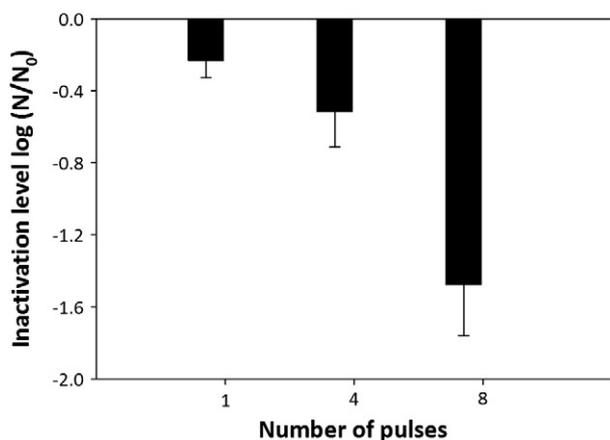
**Fig. 4.** The inactivation level of *E. coli* as a function of different numbers of 1 ms pulses at 12 kV/cm is shown. Bacterial cells (approximately 10<sup>9</sup> cells/mL) were placed in a laboratory scale continuous flow system. Pulses were applied at room temperature (22 °C). Values represent means  $\pm$  standard deviation.
