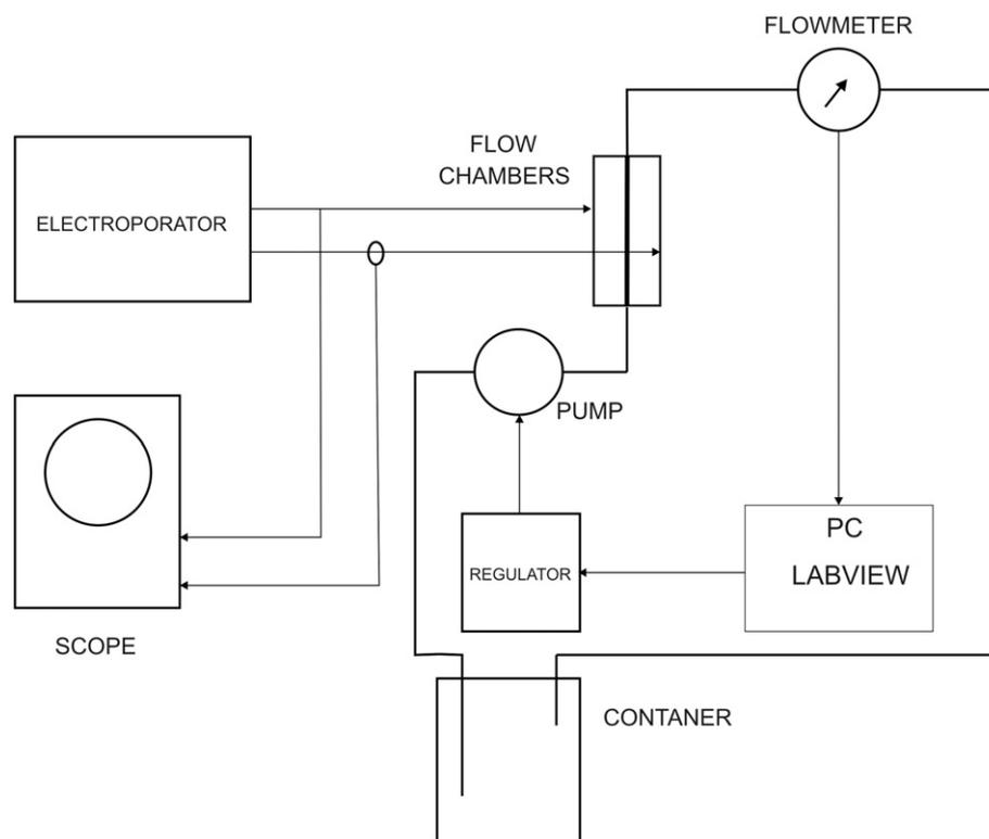
**Fig. 1.** The circuit system includes a cross-field (for bacterial cells) or co-field (for microalgae) chamber and a prototype square wave pulse generator. Voltage and current are both monitored throughout the experiment.
