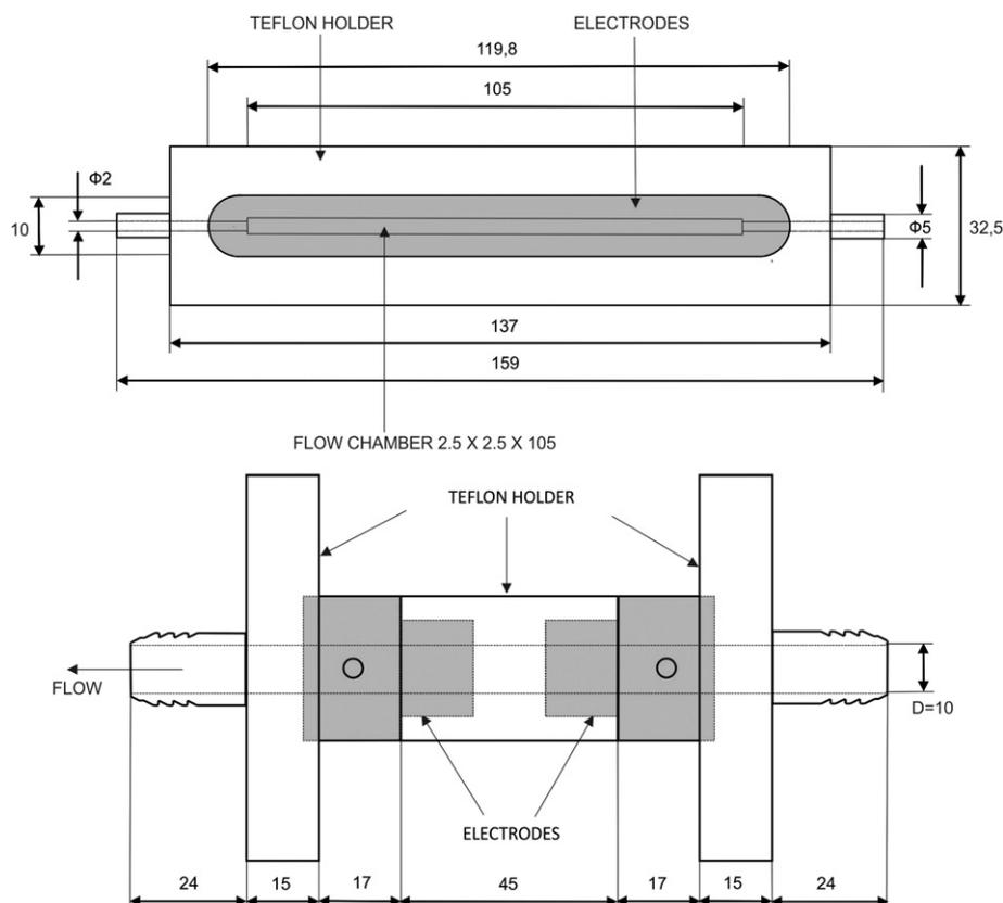
Fig. 2. Cross-field chamber (above), used for *E. coli* and co-field chamber (bottom), used for microalgae. The gray area represents metallic parts (electrodes) of the chambers.
