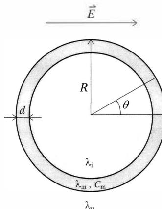
Fig. 1. The model on which the calculations were based. The cell is a sphere with radius of  $R$ . It is enclosed by a shell of uniform thickness  $d$  (the membrane). The external electric field is homogeneous, and  $E$  is the absolute value of the electric field strength vector. Specific conductivities are attributed to spaces occupied by cytoplasm ( $\lambda_i$ ), membrane ( $\lambda_m$ ) and extracellular medium ( $\lambda_o$ ). Membrane capacitance is denoted by  $C_m$ .
