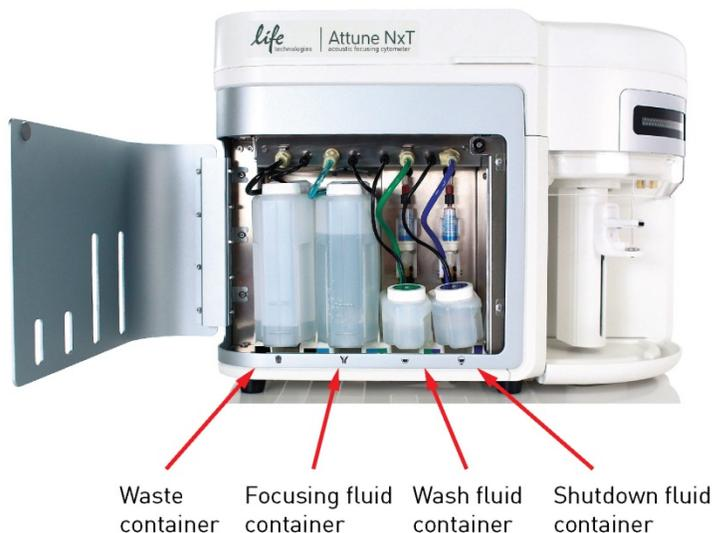
2. Fill the focusing fluid, wash solution, and shutdown solution containers (see page 21).
