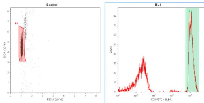
10. Repeat setup steps for the remaining compensation controls and ensure that the gates are set appropriately on the population of interest.
