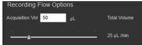
For setup, you can conserve your sample by running the cytometer at a 25 µL per minute collection rate.
