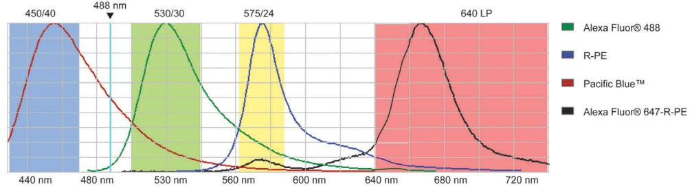
Each dye emits with a characteristic emission spectrum that is specific for the fluorophore: Alexa Fluor™ 488 dye has a maximum around 520 nm, R-PE at about 575 nm, Pacific Blue™ dye at about 454 nm, and Alexa Fluor™ 647-R-PE dye at about 666 nm. The teal line represents the laser excitation wavelength of an argon ion laser (488 nm).
