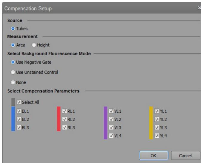
2. On the Compensation Setup dialog, select the source of compensation controls. The Compensation Setup dialog provides different options for setup based on your selection of the compensation source.
