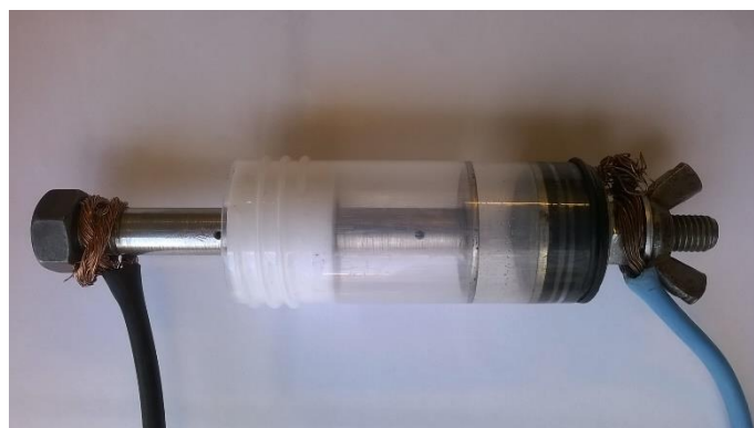
Figure 3.1: The electrical treatment chamber.
