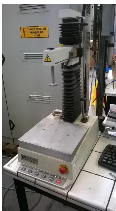
Figure 3.5: The used texture analyser TA.XT plus (image taken at the laboratory). One of the laboratory generators (an industrial-scale model, manufactured by Hazemeyer) is visible in the background.
