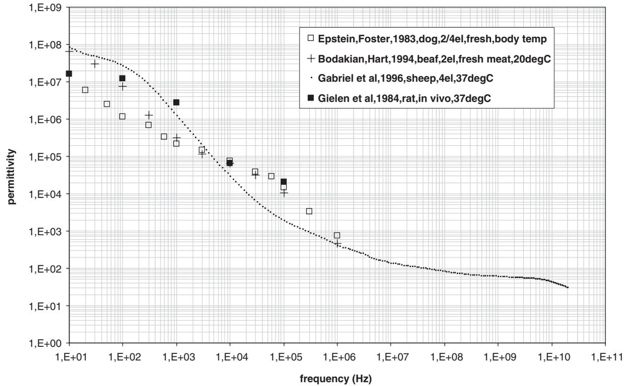
Figure 4. Relative permittivity for skeletal muscle, longitudinal direction.
