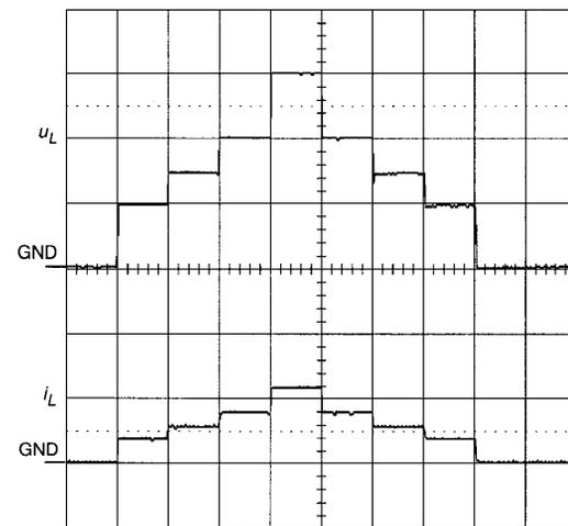
Fig. 3 Load voltage  $u_L$  and current  $i_L$  ( $k_u = 200 \text{ V/div}$ ,  $k_i = 5 \text{ A/div}$ ,  $k_t = 100 \mu\text{s/div}$ )
