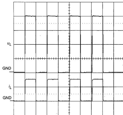
Fig. 2 Train of four consecutive pulses at 5 kHz repetition frequency, magnitude 800 V, pulse duration 100  $\mu\text{s}$  ( $k_u = 200 \text{ V/div}$ ,  $k_i = 5 \text{ A/div}$ ,  $k_t = 100 \mu\text{s/div}$ )
