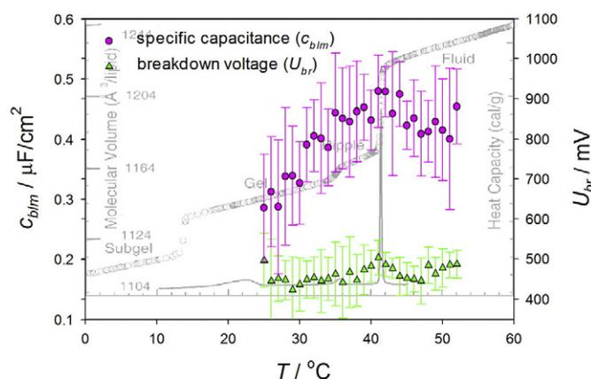
**Fig. 5.** Specific electrical capacitance ( $c_{blm}$ ) and breakdown voltage ( $U_{br}$ ) of planar lipid bilayers formed from mixture 80:20 (w:w) of DPhPC and DPPC respectively in dependence of the temperature. Measurements were done in the temperature interval between 25 °C and 52 °C. For comparison the molecular volume and heat capacity of DPPC are added [28].
