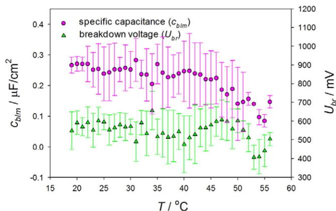
**Fig. 3.** Specific electrical capacitance ( $c_{bim}$ ) and breakdown voltage ( $U_{br}$ ) of planar lipid bilayers formed from archaeal lipids *A. pernix K1* in dependence of the temperature between 19 °C and 56 °C.
