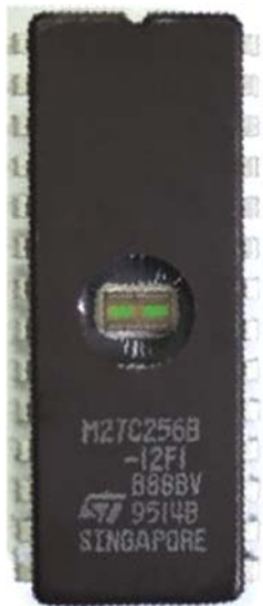
32 KB (256 Kbit) EPROM M27C256B (ST Microelectronics)
