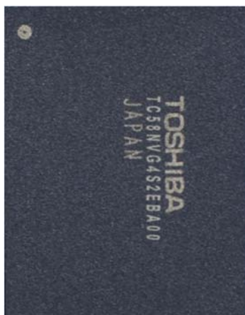
2 GB (16 Gbit) SLC NAND Flash EEPROM TC58NVG4S2EBA00 (Toshiba)
