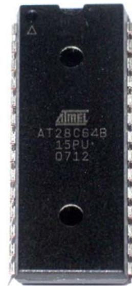
8 KB (64 Kbit) EEPROM AT28C64B (Atmel)
